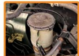
Close ball valve on yellow pressure hose and disconnect hose from master cylinder adapter. Remove the adapter and replace the master cylinder cap.
