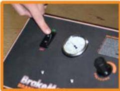
Turn the machine on and use the pressure regulator to increase the pressure to the desired amount. A typical brake service should not require more than 12psi.
