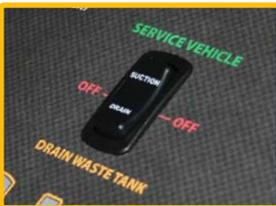
When complete, flip switch to "OFF" position.
