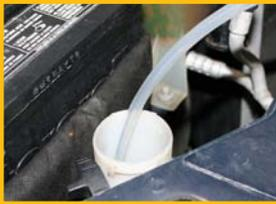
Select appropriate adapter to fit into desired fluid reservoir, and connect to machine's red service hose.
